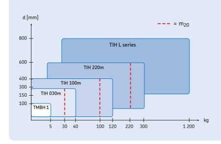
The comprehensive range of SKF induction heaters is suitable for most bearing heating applications. The chart gives general information on choosing an induction heater for bearing heating applications.<sup>2)</sup>
