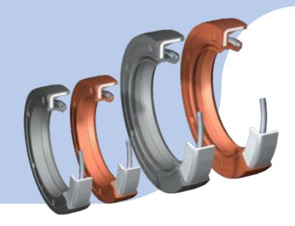
Bearing performance relies largely on the ability of the sealing system to retain lubricant and prevent aggressive contaminants from entering. Often the seals are expected to fulfill these tasks while withstanding tough operating conditions, including considerable thermal expansion, high dynamic runout and shaft-to-bore misalignment.
