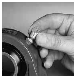
2. Place a Zerk-Lock onto the fitting
