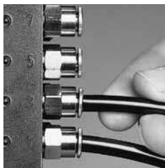
1. Install a Quicklinc into the divider valve and insert the line
