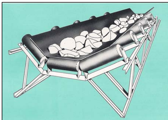
Figure 8. Heavy-Duty Conveyor (typical) [1].
